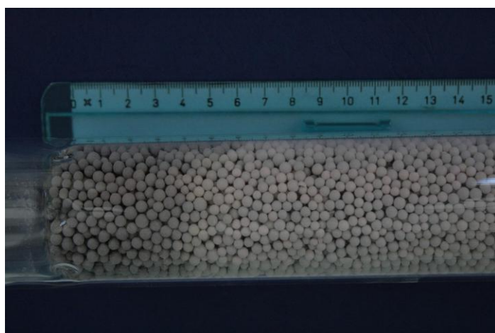
Figure 8. Fixed bed after a experimental run of 6 hours it shows a plug-flow well-rendered separation between sulphurized sorbent and fresh sorbent.
