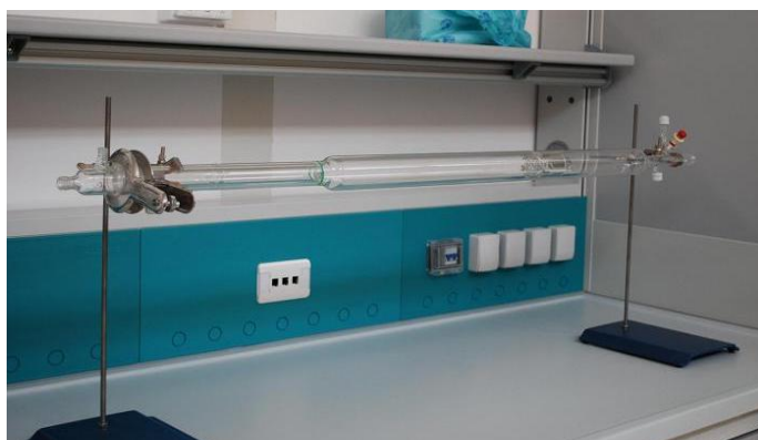
Figure 2. The experimental reactor designed by Sotacarbo and borosilicate glass manufactured for operations up to 550 °C to high temperature desulphuration H_2S removal from gaseous stream.
